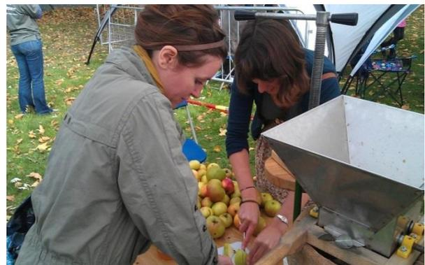
The principle equipment consists of an apple press and a 'scratter' or mill to crush the apples up into a pulp before the juice is squeezed out by the press. When choosing where to buy these look at good quality, reasonable price and their ongoing customer service after the purchase. If you plan to use your orchard produce to make juice, cider vinegar or cider then this equipment would be money well spent; an investment that will last a lifetime with care.
